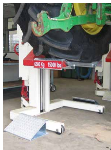
Base Frame and Lifting Fork Extensions for vehicles with recessed wheels.
