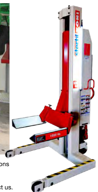
Special Pick-Up Adapters for wheel-free lifting.
