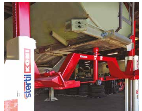
Traverse Kingpin Crossbeam for the safe and stable detachment and independent lifting of a trailer from the unit or cab.
