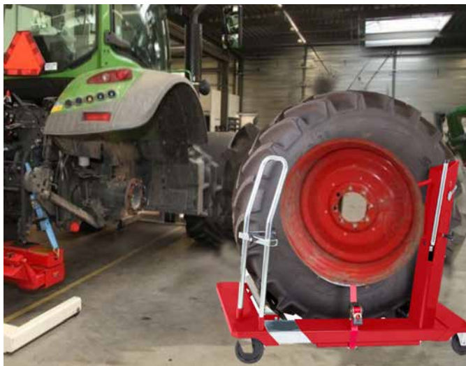
Wheel Dolly for convenient and ergonomic removal of large wheels.
