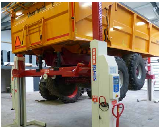
Low-Profile Crossbeam for more accessibility wheel-free maintenance.
