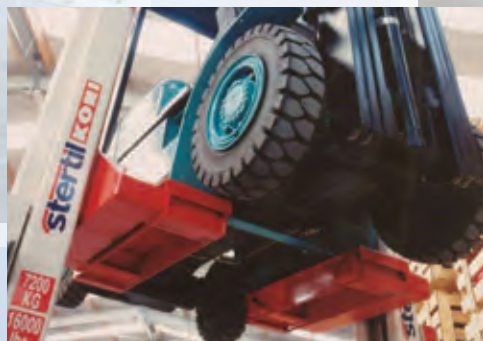
View of Four-Wheel Forklift Adapter Kit undercarriage
