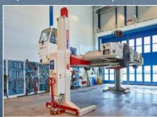
29,000 lbs per column Lifting capacity:
