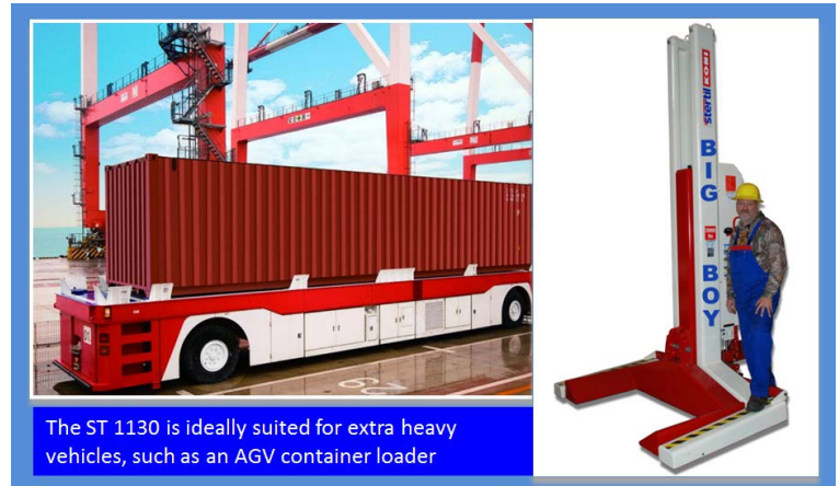
The Stertil-Koni ST 1130 mobile column lift, with a capacity of 29,000 lbs. per column.
