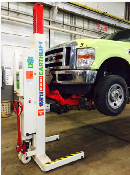
The new Stertil-Koni multi-purpose adapter is ideal for wheels free lifting, using only two mobile column lifts.
