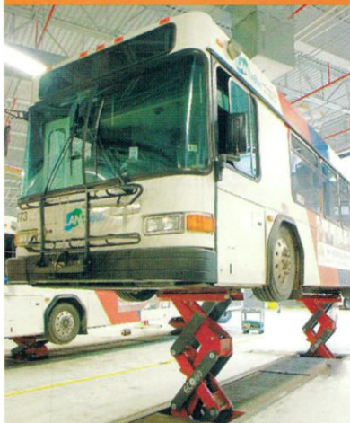
Stertil-Koni says its ECOLIFT is the industry's first, U.S. patented, ultra-shallow, full-rise axle-engaging in-ground scissor lift.
