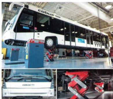
The ECOLIFT's total lifting capacity is 30,000 pounds per scissor.
