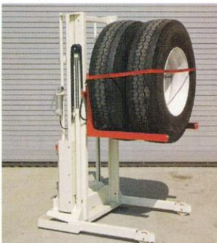
The high lift wheel dolly lowers the occurrence of back injuries and abdominal strains because wheel removal is completed at an altitude in line with technicians working in a fully standing position.
